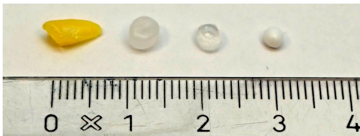
Figure 1: Plastic pellets analysed in the project, from left to right: PE-HD ( \approx 5 mm), PE-LD ( \approx 4 mm), PP ( \approx 3 mm) and PET ( \approx 2 mm).
