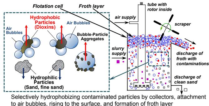
Figure 2: Contaminant removal in flotation process
