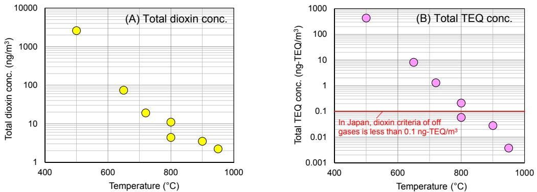
Figure 5: Total dioxin/TEQ concentrations of the gas samples in the temperature range 500 to 950°C
