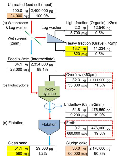
Figure 4: Process route of soil-A treatment
