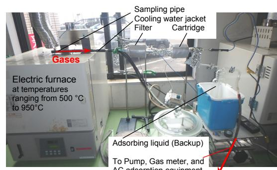
Figure 3: Laboratory test system of incineration
