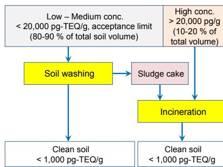
Figure 1: Combined use of soil washing and incineration
