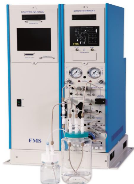
Figure 1. Automated Solid Phase Extraction System for Perfluorinated Compounds and PPCPs.
