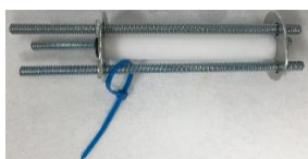
Figure 2. Photograph of the PE passive sampling device contained within metal deployment apparatus.
