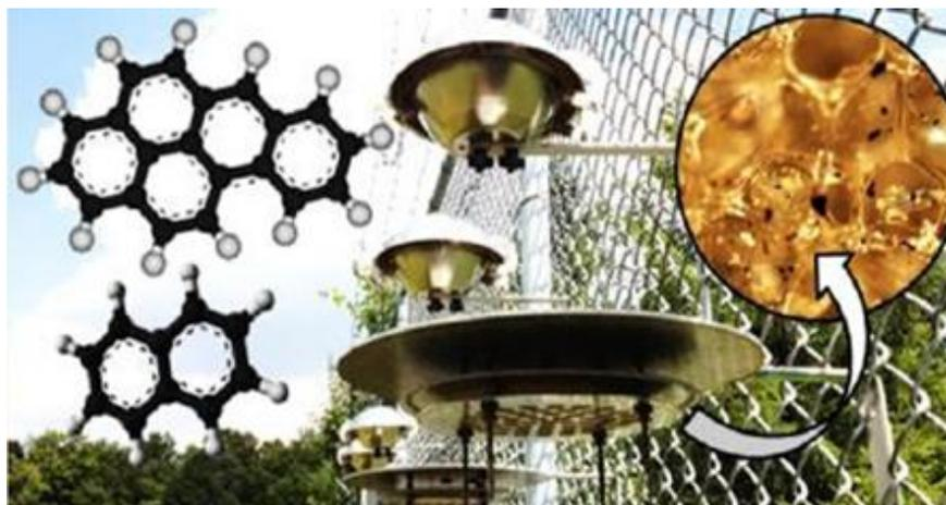
Figure 1. Illustration of the PAS-DD sampler (bottom) and the PUF disk sampler for assessing priority chemicals in air (from Eng et al., 2014).
