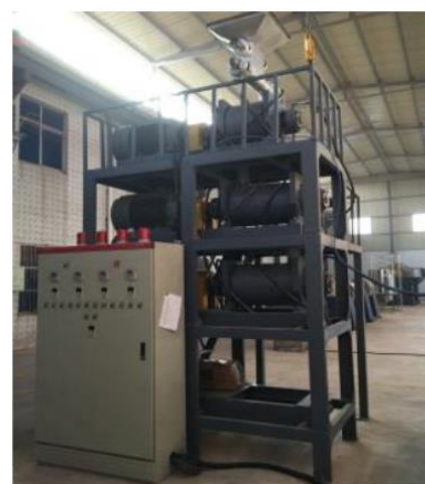
Fig. 2 Appearance of multi-level successive high-energy mill
