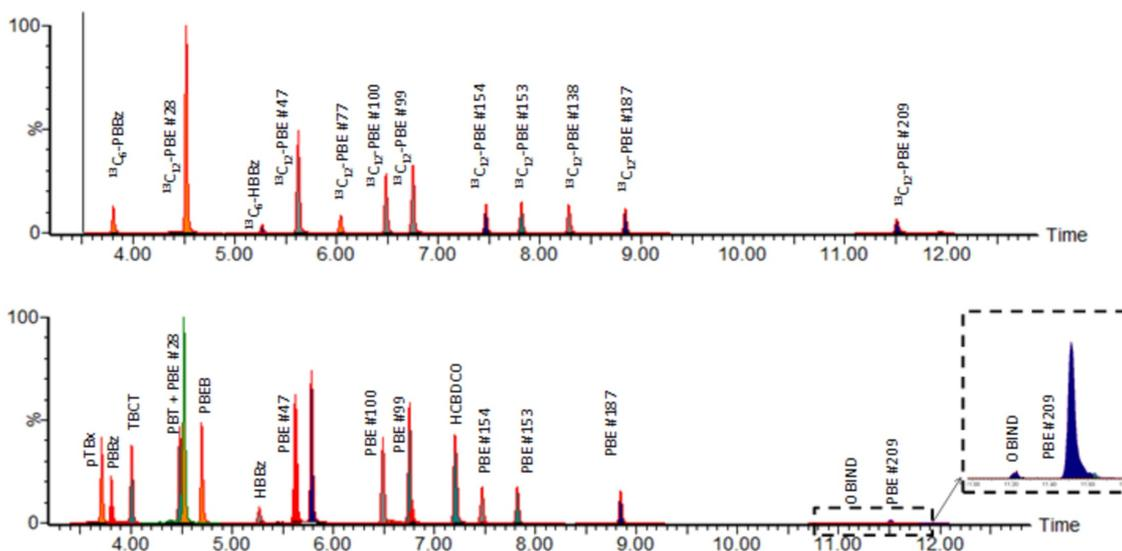
Figure 2: Diagnostic GC/APCI/MS/MS ion chromatograms obtained for labeled (top) 25 pg injected except 50 pg for  $^{13}\text{C}_{12}$ -BDE #209 (split 1:5; 5 pg and 10 pg on-column respectively) and native BFRs (down) 100 pg injected except 50 pg for BDE #209 and O BIND (split 1:5; 20 pg and 10 pg on-column respectively)
