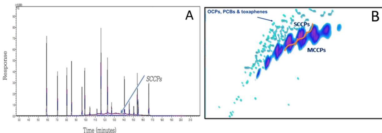
Figure 1: A) Total ion chromatogram of polychlorinated compounds (organochlorine pesticides (OCPs), polychlorinated biphenyls (PCBs) and SCCPs 63% Cl content by weight) and B) GCxGC-ECD contour plot of MCCPs 57% Cl (below orange line) and SCCPs 63% Cl (above orange line), as well as polychlorinated compounds (OCPs, PCBs and toxaphenes), indicated by blue dots.
