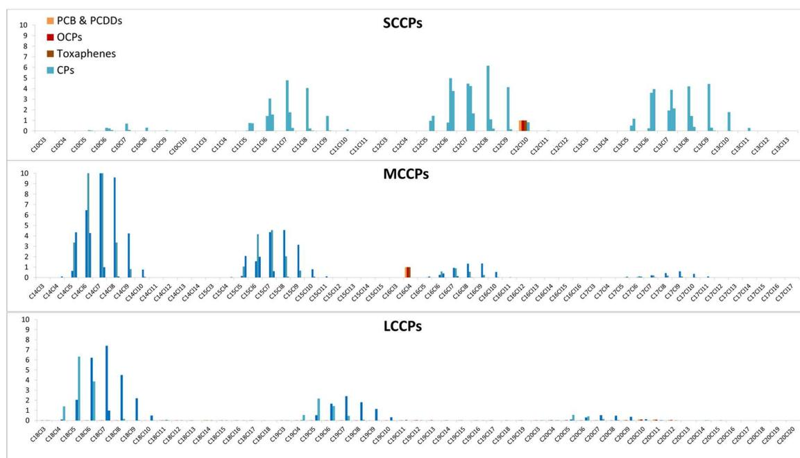
Figure 2: Measured response of CP mixtures and other polychlorinated compounds (e.g. PCBs, OCPs, PCDDs and toxaphene) on nominal masses from CP congener groups measured by  $\text{CH}_2\text{Cl}_2$ -APCI-QTOF-M.
