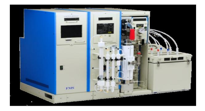
Figure 1. Automated cleanup system, PLE, and evaporator.
