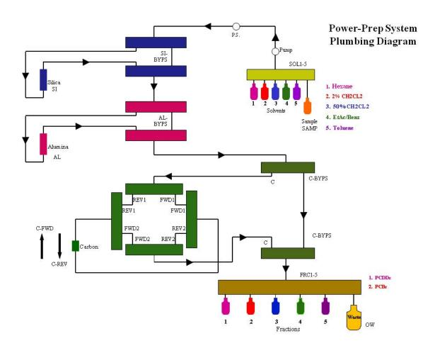
Figure 1. Automated Column Chromatography System Schematic.
