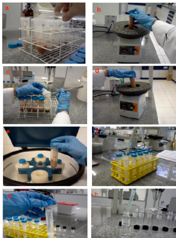
FIGURE 1 – Extraction of the POPs by QuEChERS method from the industrial region soil.
