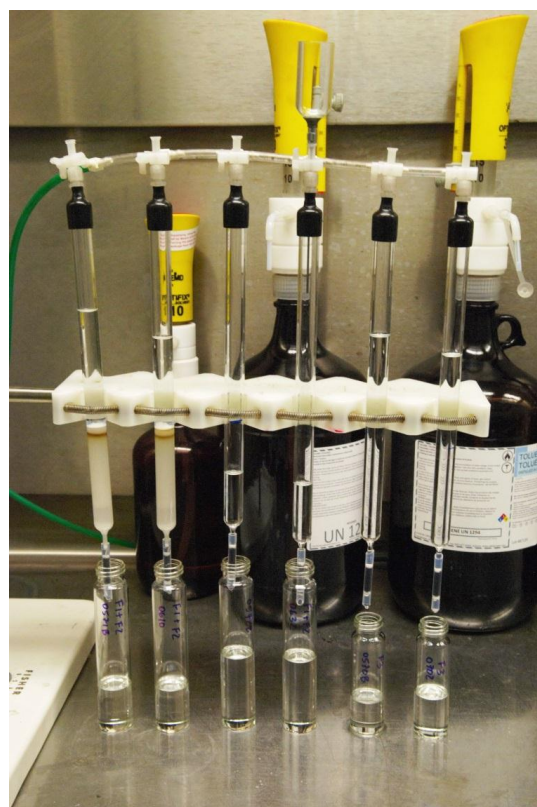
Figure 1. Cape Technologies tandem acid silica / carbon columns collecting F1, F2 and F3
