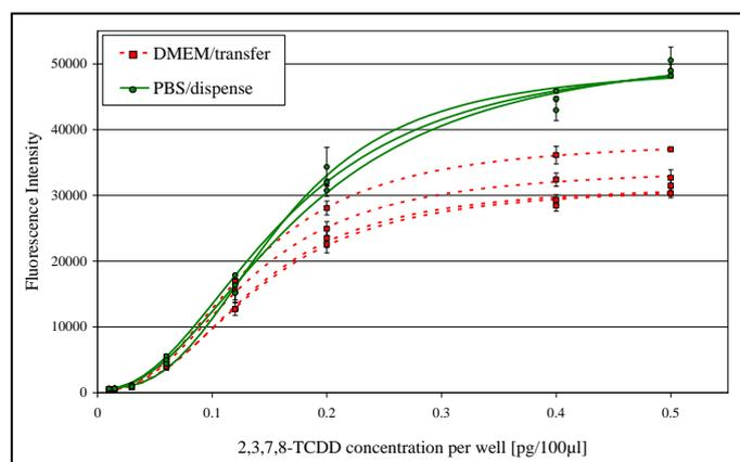
**Figure 1:** Test of substrate handling, each data point represents the mean of three wells. Error bars are SD of triplicates. Green slopes and circles are data of plates with ETX in PBS and methanol added to the wells (PBS/dispense). Red squares and lines represent the former routine (DMEM/transfer) ETX in DMEM and transfer to a second plate. Results of relevant curve parameters (mean ± SD) were:
