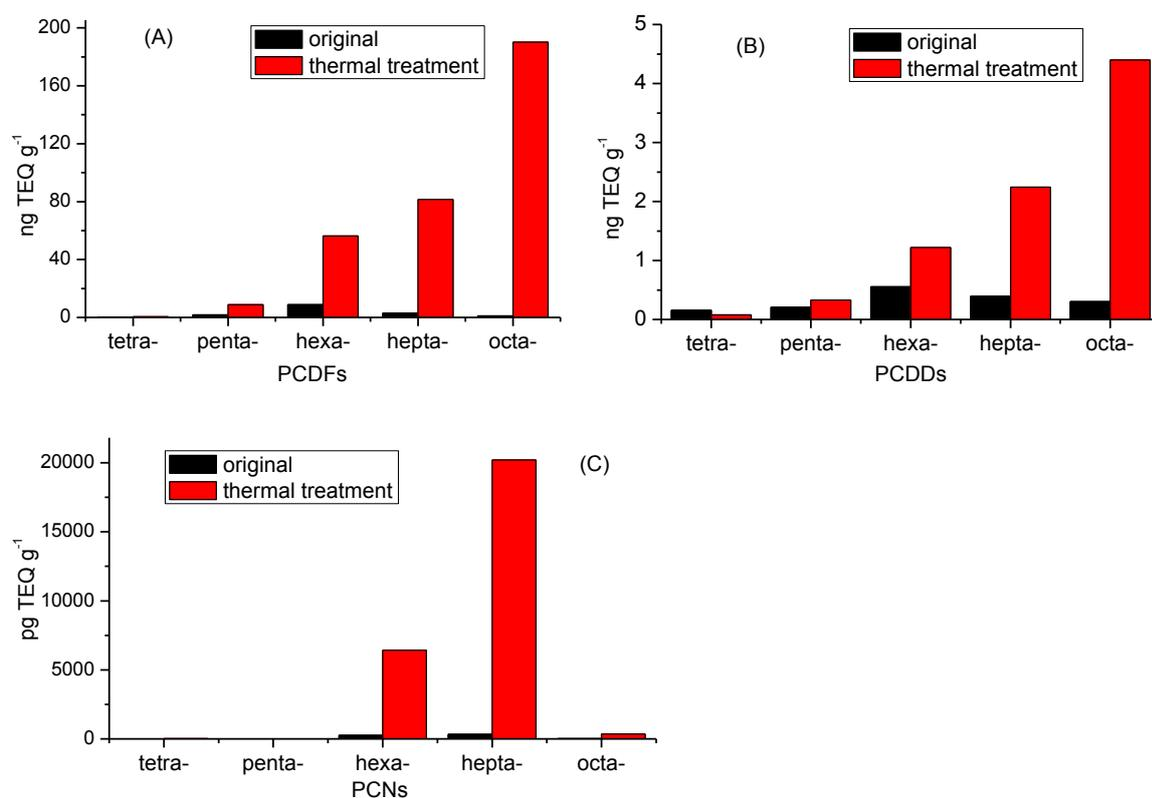
Fig. 1 TEQ increments of PCDFs, PCDDs, and PCNs after thermal treatment of fly ash in tube furnace
