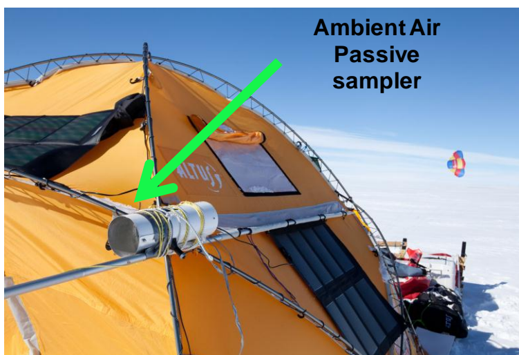
Figure 1. Scheme and passive sampler attached to the wind-driven sludge
