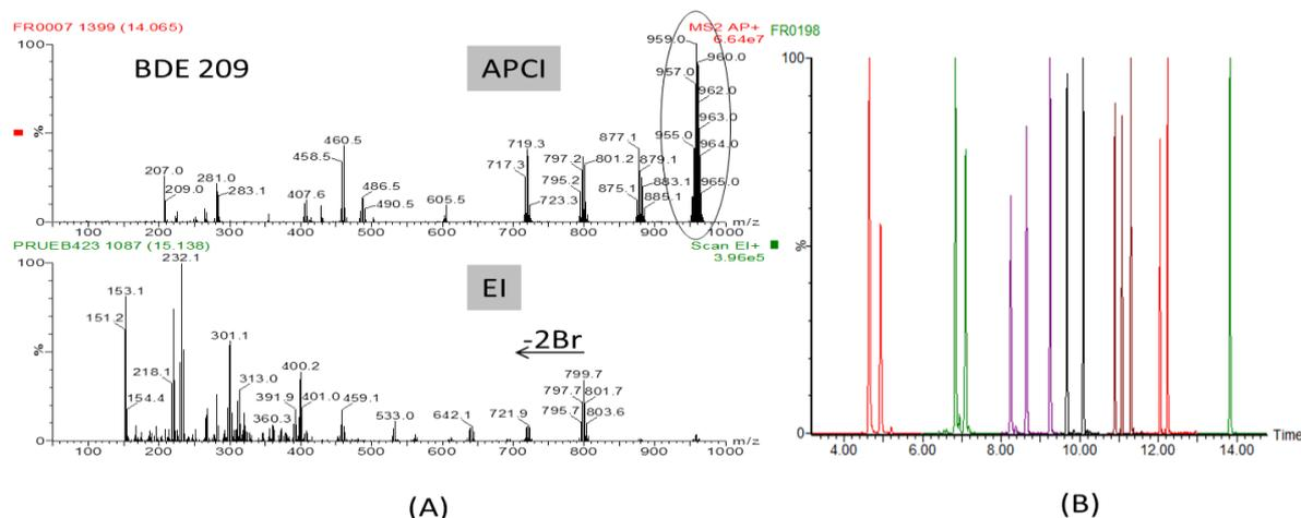
Figure 1. (A) APCI (up) and EI (bottom) spectrum of BDE 209. (B) GC-(APCI)MS/MS overlay SRM chromatograms for the lowest calibration level injected ( $1 \text{ ng mL}^{-1}$  for  $Br_{3-8}$  BDE and  $5 \text{ ng mL}^{-1}$  for BDE 209)
