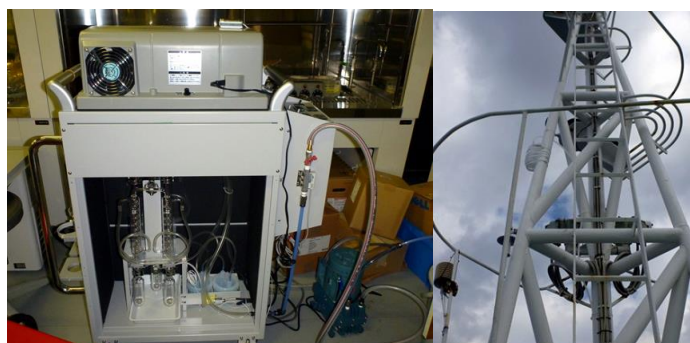
Figure 1. Cryogenic Moisture Sampler (CMS type 1st) in a laboratory and inlet system on board.
