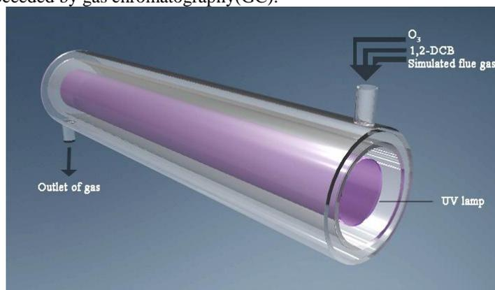
**Fig.1** The schematic diagram of the quartz reactor
