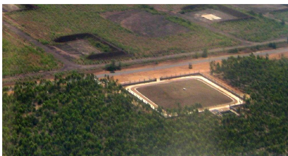
Photo 1 Aerial View of Newly Completed Containment Landfill in Phu Cat (45m x 45m)
