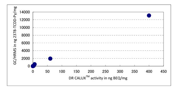
**Figure 2:** Comparison of dioxin-like activity measured by DR-CALUX<sup>TM</sup> (in ng BEQ/mg) and concentrations for the sum of cis/trans 2,3,7,8-TCDD-py by GC/HRMS (in ng/mg) of thermally treated chlorpyrifos, chlorpyrifos-methyl and 3,5,6-trichloro 2-pyridinol standards. (**please note:** the uncertainty in the measured 2,3,7,8-TCDD-Py concentration using 2,3,7,8-TCDD standard).
