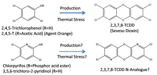
**Figure 1:** Formation of 2,3,7,8-TCDD from 2,4,5-T/2,4,5-TCP and potential formation of the 2,3,7,8-TCDD pyridine analogue from Chlorpyrifos or 3,5,6-trichloro-2-pyridinol (used in Chlorpyrifos production).
