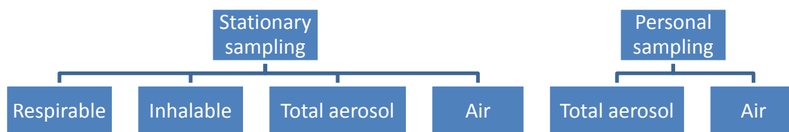
Figure 1 shows the particulate (respirable, inhalable and total aerosol) and air fractions collected in stationary and personal sampling.
