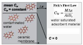
Figure 1. Concentration profile in the ceramic toximeter.
