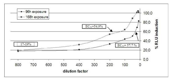
Figure 3. An overview of the dilution curves for two ceramic dosimeters with exposure times of 96 and 168 h
