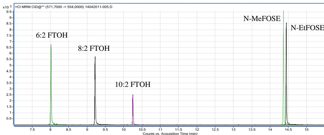
**Figure 1:** typical diagnostic ion chromatogram obtained in GC-(CI+)-MS/MS for the five perfluoroalkyl precursor compounds analysed (0.02 ng injected on-column).
