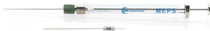
Figure 1. The MEPS syringe and SPE cartridge or BIN “ B arrel I nsert and N eedle” filled with 2 mg of sorbent commonly used for SPE.
