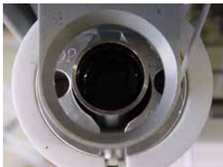
Figure 6. Bad positioning of the cell in the PLE heating element
