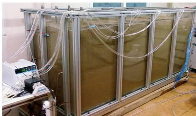
Figure 1. Pilot test was conducted in a sandy media packed box (2m x 1m x 0.75m, L x H x W)
