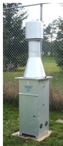
Figure 1. Photo of the SHV air sampler equipped with XAD-2-impregnated PUF disks
