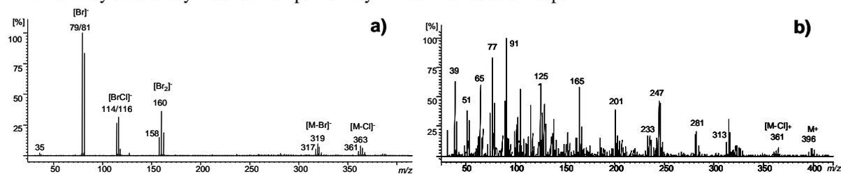
Figure 2: Mass spectra of MHC-1 as recorded in the (a) GC/ECNI- and (b) GC/EI-MS modes
