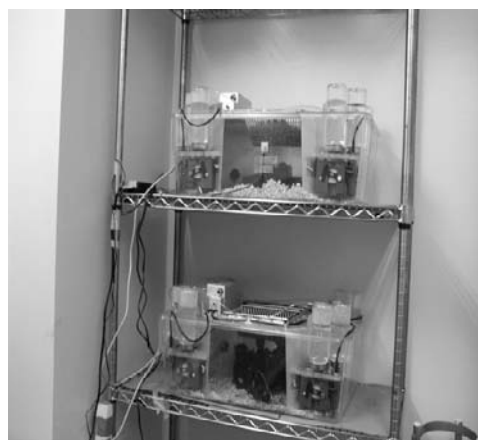
Fig. 2. IntelliCage, an automated system designed for continuous long-term recording of the home cage behavior.
