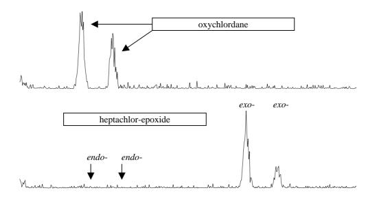
Figure3 GC/MS-SIM chromatogram showing elution of heptachlor-epoxide (average of m/z 352.8442 and 354.8413) and oxychlordane (average of m/z 386.8052 and 388.8023) on BGB-172 HRGC column in serum sample.
