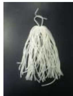
Photo 1 A passive sampler made of yarn
