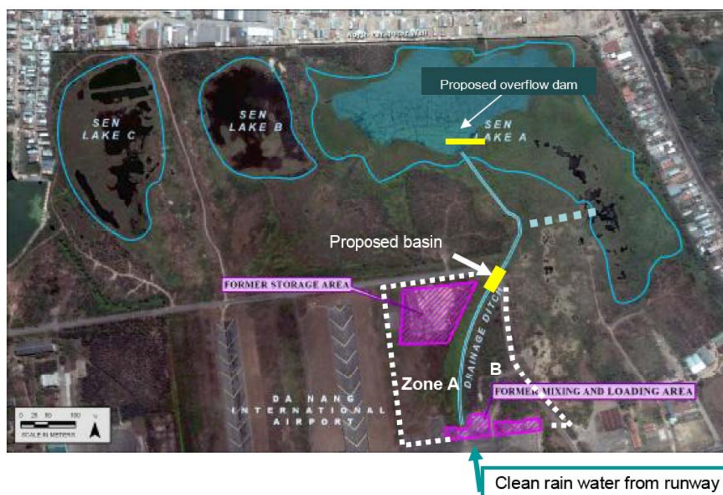
Mitigation measures for the mixing loading and the former storage area
