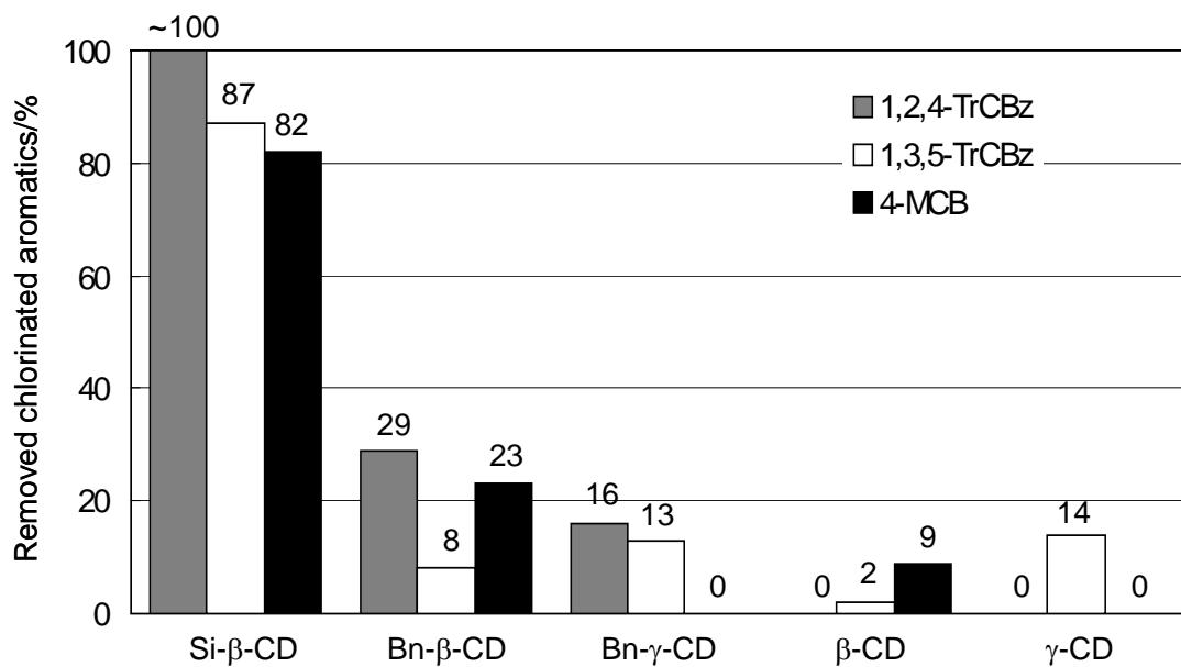
**Figure 3.** Percentage of chlorinated aromatics removed from insulating oil after stirring with various types of CD derivatives for 15 h at 25 °C. Initial concentrations of chlorinated aromatics in insulating oil were 90 ppm. The amounts of CD derivatives added were 20 mg.
