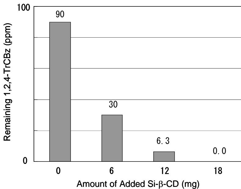
**Figure 4.** Relationship between the amount of 1,2,4-TrCBz remaining in insulating oil (242 mg) and the amount of added Si- $\beta$ -CD. Initial concentration of 1,2,4-TrCBz was 90 ppm.
