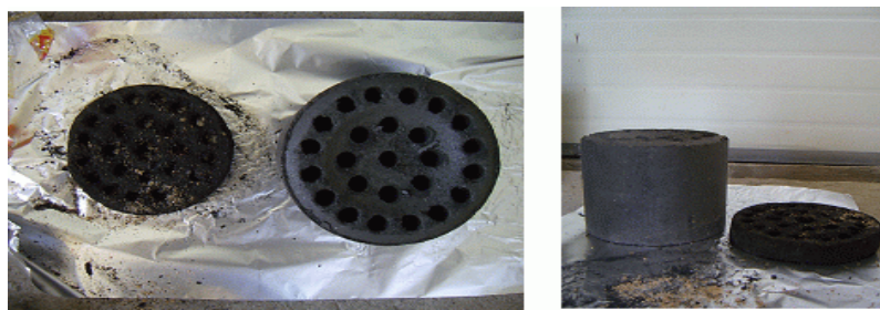
Fig.1. Ignition Briquette and Briquette used as a fuel for the house heating.
