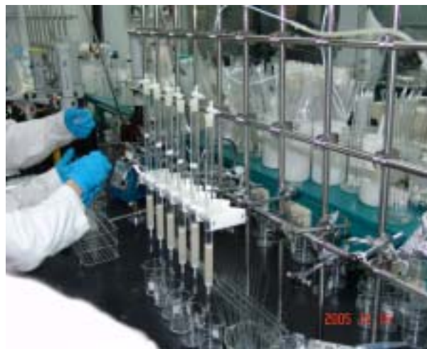
Fig. 2: CAPE coupled carbon-acid silica column
