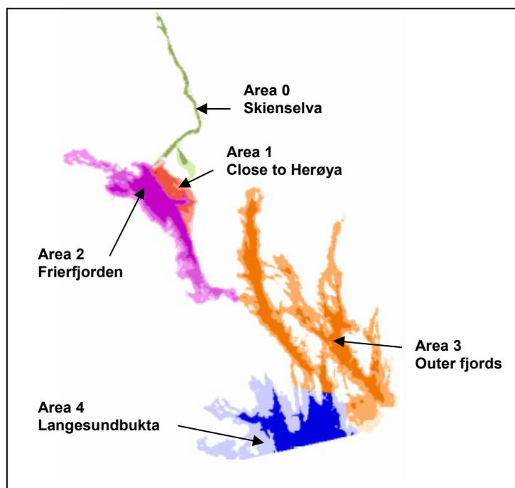
Figure 1. A bathymetric map showing the basis for horizontal compartment division in the model application for the Grenland fjords. The different colours show the horizontal division to five compartments, while the shading within a colour indicates the different bottom depth intervals used in the vertical compartment division.
