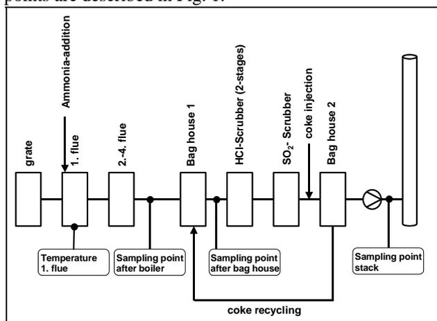
Fig.1: plant scheme and sampling locations
