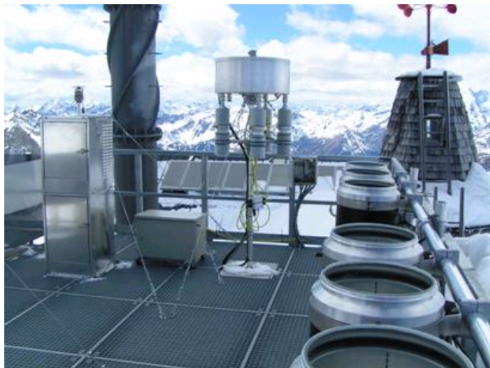
Figure 2: MONARPOP air and deposition sampling station at the Sonnblick, 3106m above sea level (Austria)
