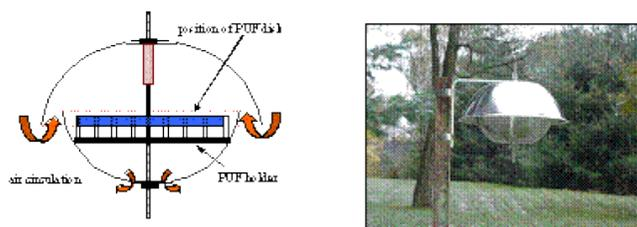
Figure 1. Schematic and photograph of PUF disk passive air sampler.
