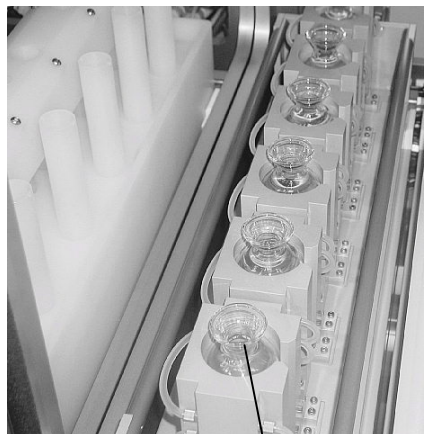
Photo.-1 Concentrator for sample (hexane solution) after H_2SO_4 treatment
