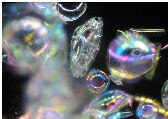
Fig. 1 Optical microscope image of microballoon formed from the FWG in a hot wind.
