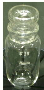
Figure 1. 80mL centrifuge-tube. Liquid-liquid extraction was done, and a water layer and an organic layer are separated in one centrifuge-tube.
