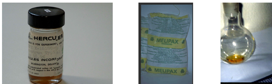
Figure 1: Photos of the technical products analyzed. Left: US-American product Toxaphene (Hercules Inc.), center: Former East-German product Melipax (powder, 10% content of active pesticide), right: Melipax waxy oil extracted from powder.
