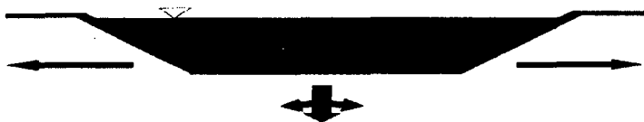
Fig 2 – Canal section: Potential dispersion of the pollutants.
