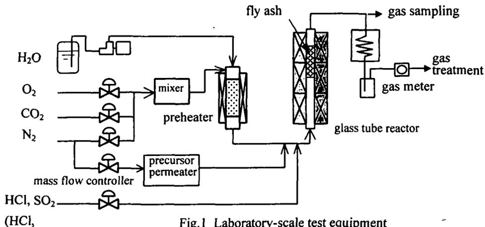
Fig.1 Laboratory-scale test equipment
