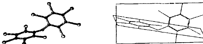
Figure 5. Two different representations of the orthogonal confirmation of DBDPO. Both images show DBPDOs aromatic rings are arranged in space at a 90 degree angles with a bend at the ether linkage.
