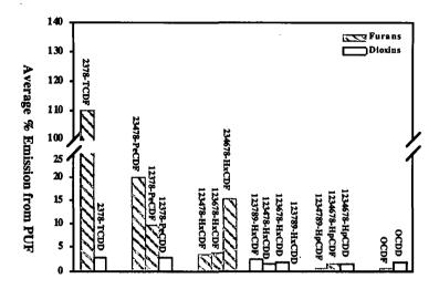
Figure 1. Average percent emissions of dioxin/furan congeners from PCP-treated wood samples after combustion at 580-720° C.
