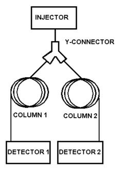
INJECTOR 1 INJECTOR 2 COLUMN 1 COLUMN 2 Y-CONNECTOR MASS DETECTOR
