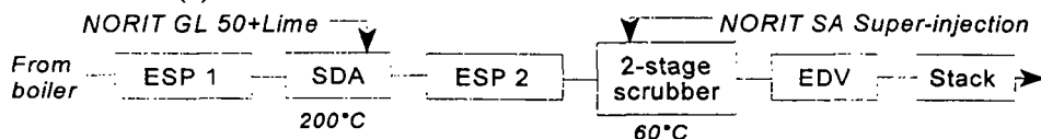
Figure 2 Schematic representation of the flue gas cleaning installation of Incinerator B. Incinerator B consists of four municipal waste incineration lines, producing 165000 Nm 3 /h flue
