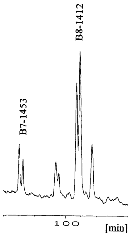
Figure 3: GC-ECD chromatogram (part) of the enantiomer separation of B8-1412 and B7-1453 in grey seal blubber on \beta -TBDM GC oven program: 120°C (2 min), 15°C/min to 140°C (150 min), 20°C/min to 220°C (10 min)
